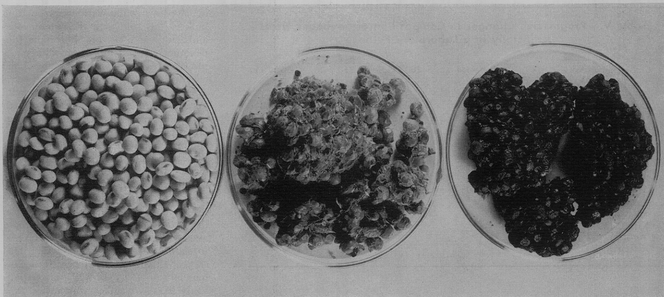
Figure 1. Typical appearance of soybeans at progressive stages of advanced spontaneous heating
